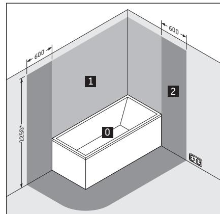
\* or the height of the highest shower head / water outlet that is permanently installed, depending on which is higher
